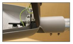
11. Make sure that the luminaire is correctly horizontally installed. Tighten two Allen screws with tightening torque of 8 Nm and secure with nuts
