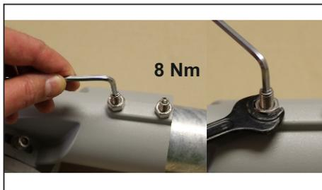
18. Loosen two imbus screws to set an angle of the luminaire. Tightening torque of 8 Nm.
