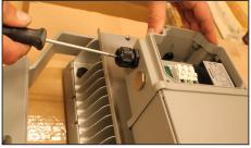
9. wiring - 2 core cable. Recommended cable -rubber cable H07RN-F 2Dx1mm2
