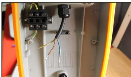
12. Connect wires to the disconnecter.
