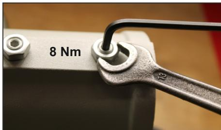
18. Loosen two allen screws to set an angle of the luminaire. Tightening torque of 8 Nm.
