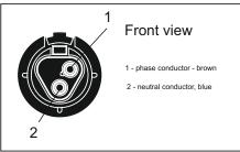
2a. Prepare the luminaire for the instalation. With a connector gesis.
