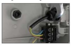
11. Strip the end of the cable (7 cm) and the ends of the wires (1 cm)
